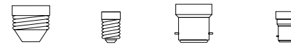
Large screw fitting (ES) Small screw fitting (SES) Large bayonet fitting (BC) Small bayonet fitting (SBC)
